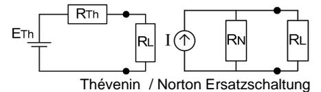
$$R_{Th} = R_N \quad I_N = \frac{E_{Th}}{R_{Th}} = \frac{E_{Th}}{R_N}$$
